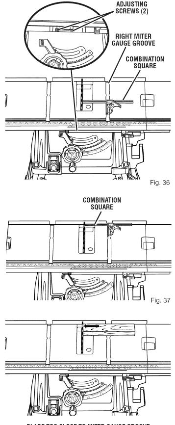
**BLADE TOO CLOSE TO MITER GAUGE GROOVE**
